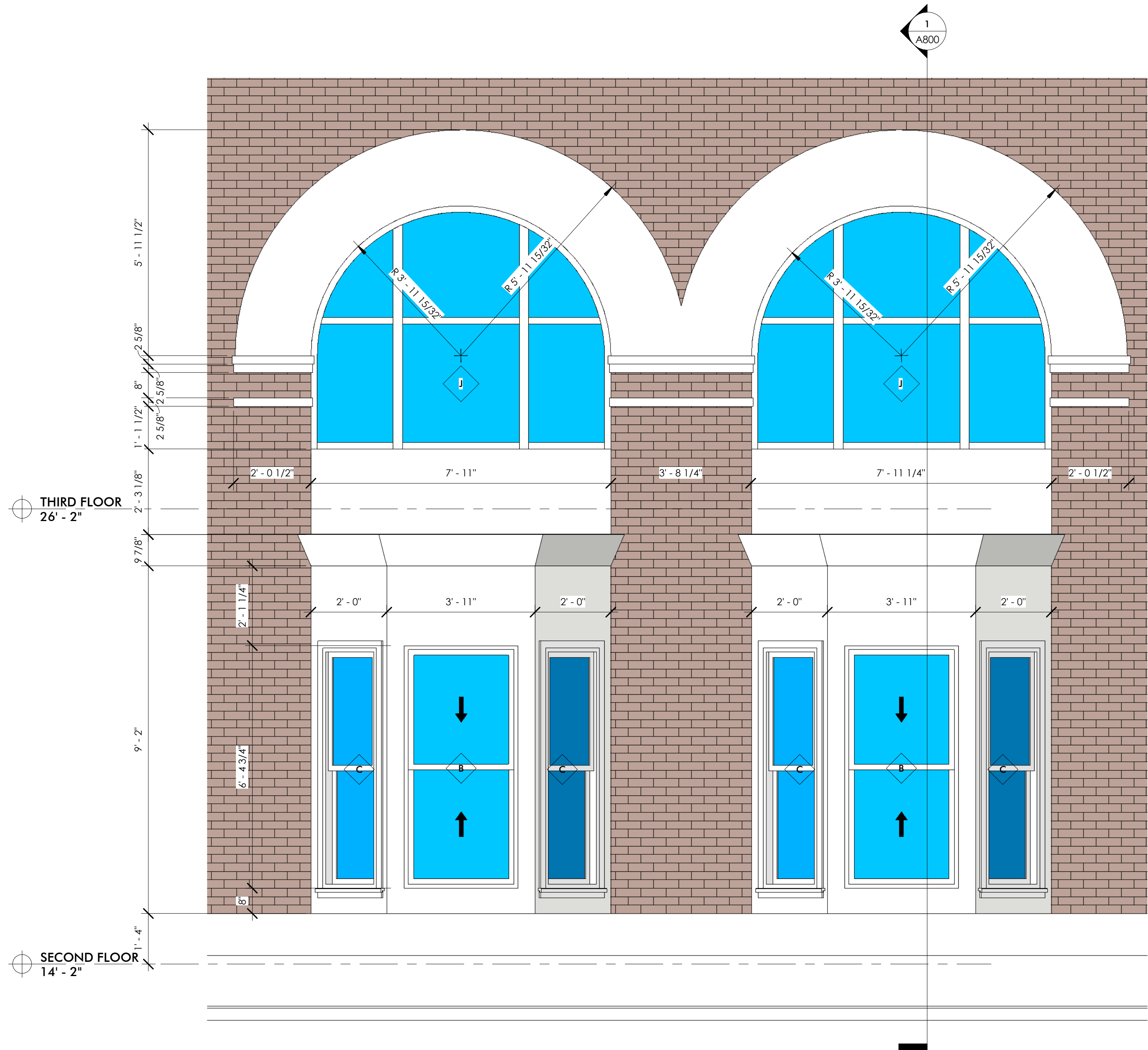
3 NORTH ELEVATION DETAIL 1/2" = 1'-0"
